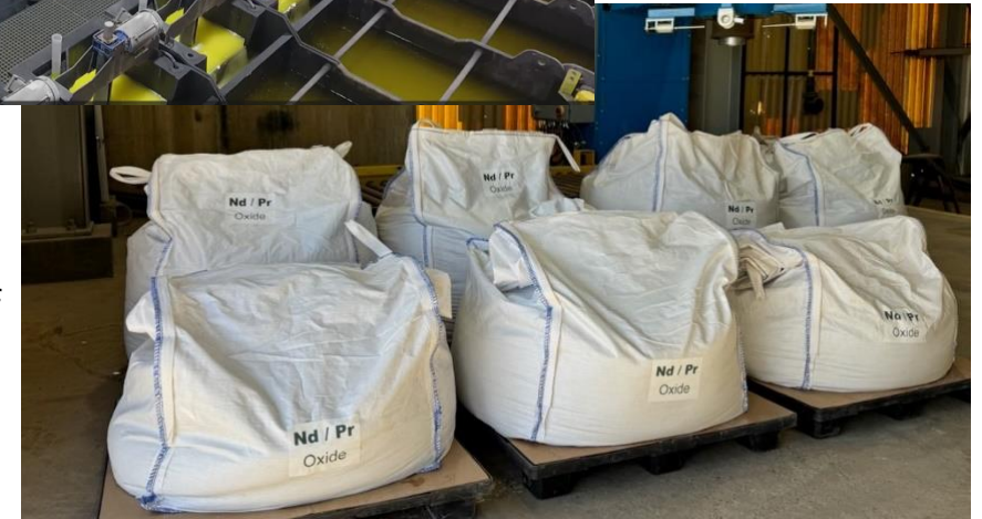
One (1) tonne "supersacks" of NdPr oxide produced at the White Mesa Mill
