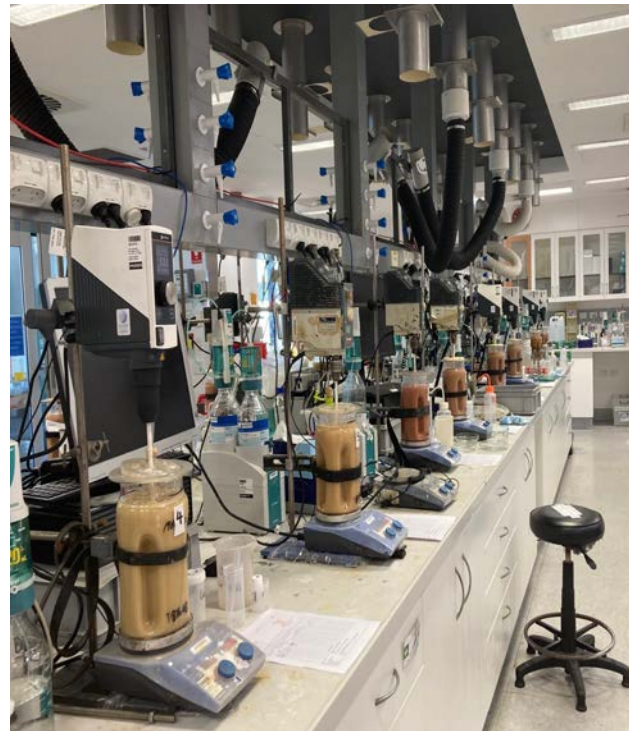
Diagnostic leach tests being conducted in the ANSTO Minerals Leach Laboratory, Sydney, NSW
