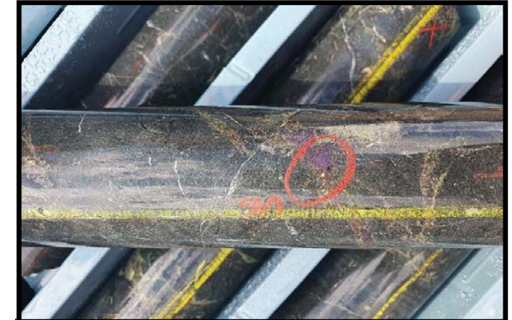
Hydrothermal (bornite-chalcopyrite-magnetite-actinolite-calcite) cemented breccia at Kaiser KAI -161m @ 0.38g/t Au, 0.47% Cu incl 27m @ 1.29g/t Au, 1.20% Cu and 7m @ 0.49g/t Au, 0.74% Cu%
